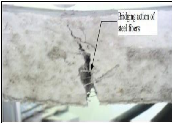
Figure: beam Specimen with steel fibre
